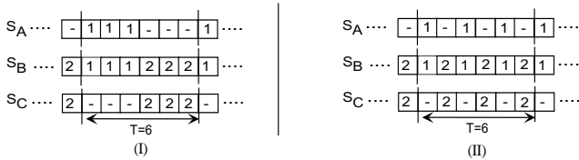
(b) Synchronized system: Two possible synchronized schedule instances realizing slot allocation (\tau_1, \tau_2) = (3, 3) in a minimum period of 6 slots
